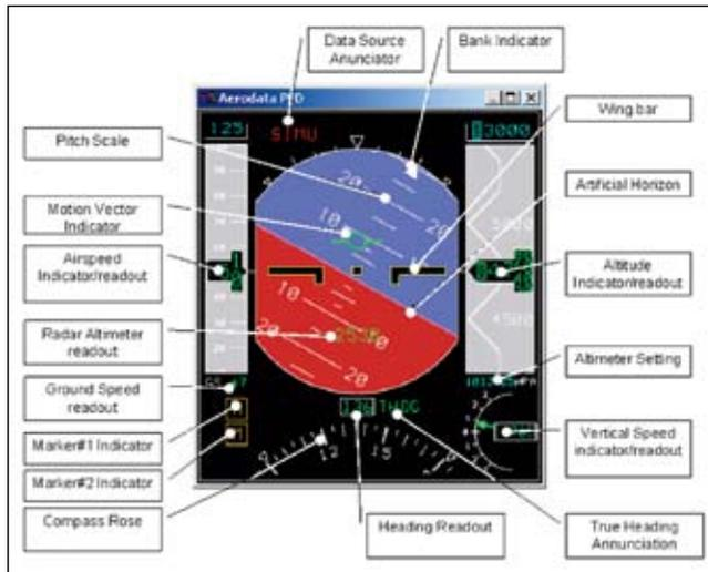
FIGURE 6 Example of the artificial horizon display of AeroMission
