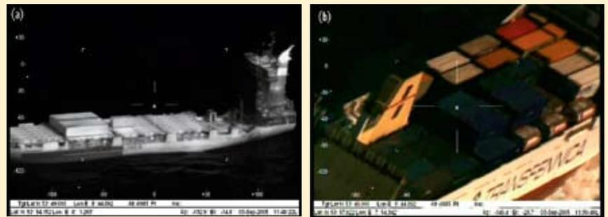
FIGURE 4 Example of the FLIR display: infrared (a) and visible band (b)
