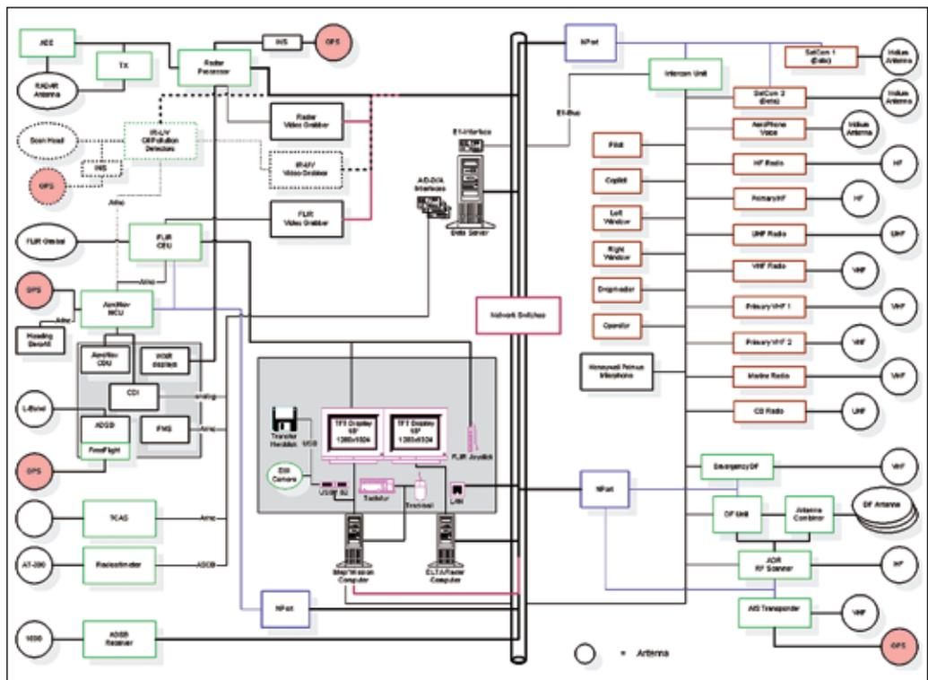
FIGURE 1 Block diagram of AeroMission (GPS antennas are marked red)
