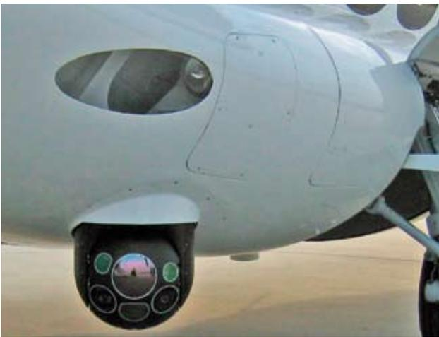
The turret of the electro-optical/infrared sensor
