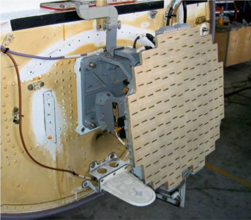
Nose-mounted surveillance radar antenna
